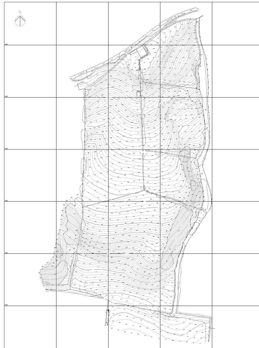
Fig. 3.5: Topographic survey of application site
